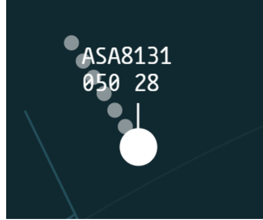
Fig. 7: Example of an aircraft displaying false altitude. The aircraft has just entered the airport area and the left value shows altitude of 5000 feet.
